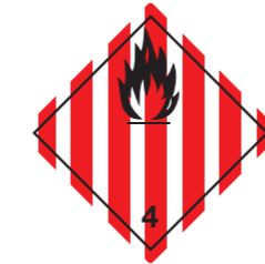
substances solides inflammables no symb. 400
